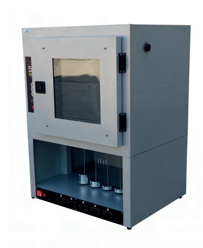
USED TO TEST STRENGTH OF ADHESIVES
